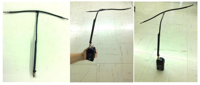
**Double Bazooka V2** (version 2) is ultimate Portable Antenna made by Batos RTV which gives you **Portability**, **Communication Distance** and **Convenience** with a gain of just over **4.2dBi** at a **reasonable** price (it will give you up to +9dB more gain against **most** of the original rubber ducks supplied with the portable sets).
